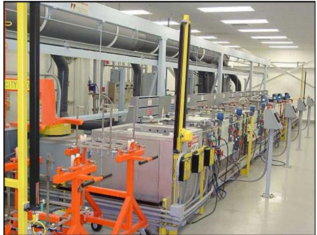
Fig. 20 Platinum electroplating line, semi-automated
