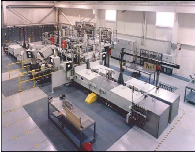
Fig. 23 A 4-chamber EB-PVD production coating system
