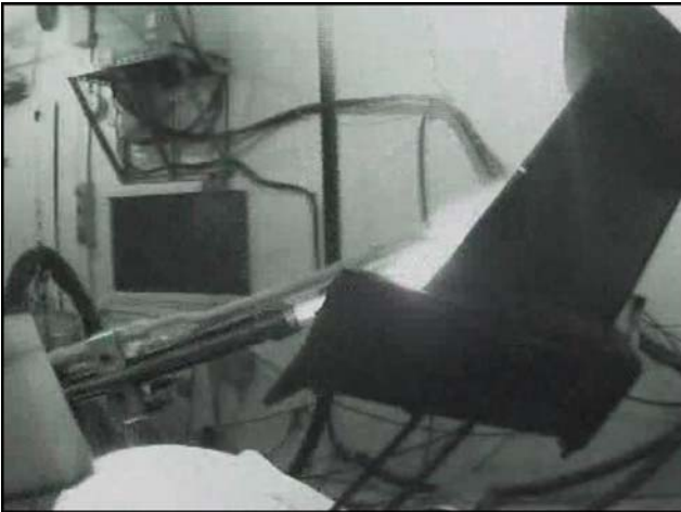
Fig. 18 A large IGT vane, with the trailing edge receiving an HVOF applied bond coating
