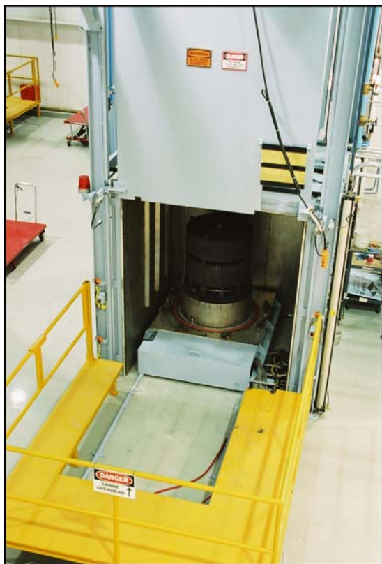
Fig. 21 VPA aluminizing furnace
