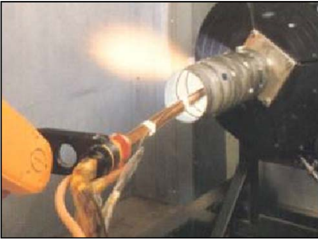
Fig. 13 Plasma TBC coating of an annular combustor
